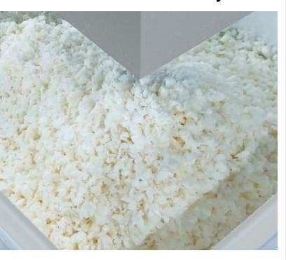
Deville Technologies' hygienic FS40 shredder is perfect for reducing coconut oil. Unlike centrifugal shredders, the oil will not heat up while operating the equipment. Shredding or crumbling a full block of coconut oil in 20-30 seconds is easy!
